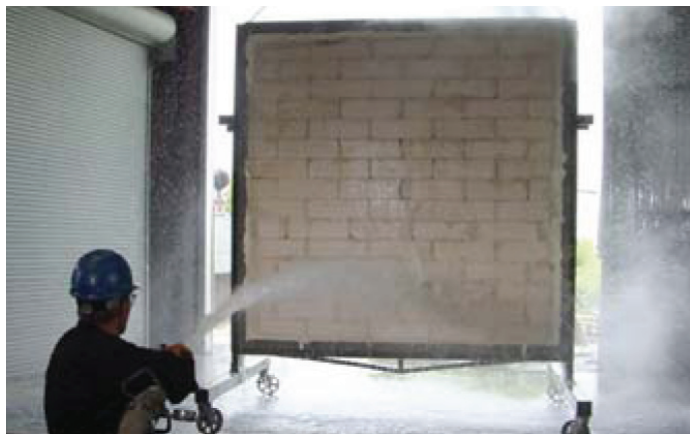
AAC has passed both the Fire Test and Hose-Stream Test sections of ASTM E119.
